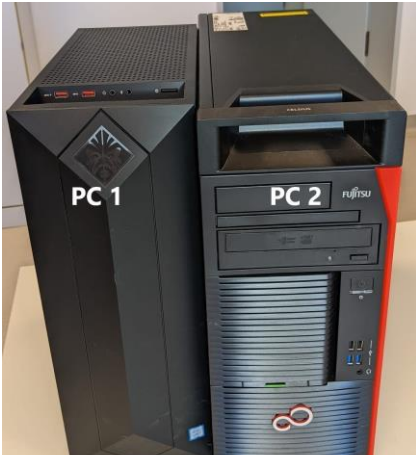
a) 5G Core Computer (PC1) and 5G-RRU (PC2) Fig. 3. Private 5G SA system hardware.
