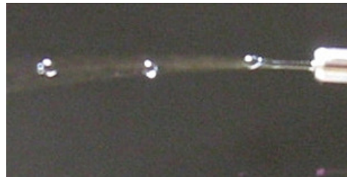
High speed imaging (100 fps). Dispensing of DI water using a 250 \mu\text{m} nozzle
