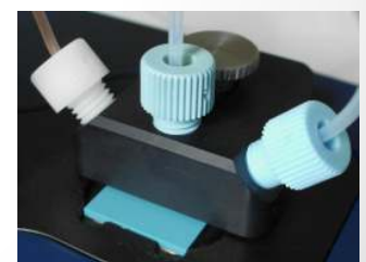
chip holding system with micro reaction chip inside
