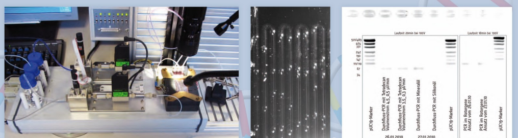
Fig. 4 Part A of the figure shows the setup used for continuous PCR on a chip. A Peltier heating element is placed under the chip, controlled by a heating system. Three temperature zones are created, the sample flow over those temperature zones is volume flow controlled. Part B shows the view through the camera positioned above the PCR-Chip. Sample drops are of equal size, spaces generated by carrier fluid do vary a little. Part C shows the image of an agarose gel of PCR products generated by continuous PCR on a chip. On the left side samples of different volume flows in line 2 and 3 and of different carrier fluids in line 4 and 5 were separated, on the right side reference samples amplified in a regular PCR-apparatus are shown as positive controls of the PCR-process.
