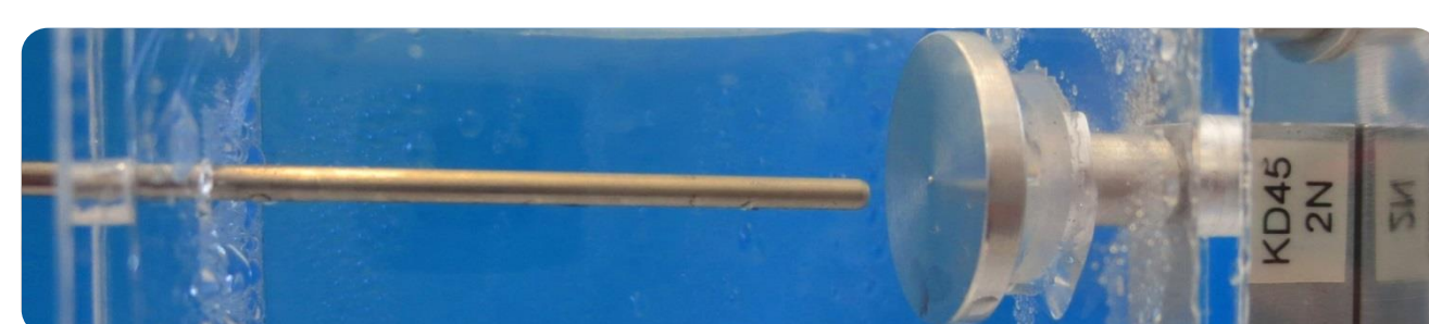
Fig. 6. Nozzle of a WAL-cannula in front of sensor head; the curved plate was removed before measurement
