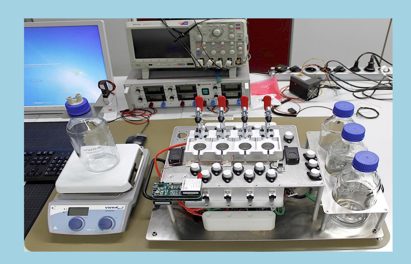
Model overview: The microGUT model is an automated desktop-sized microfluidics-based model of the human gastrointestinal tract (GIT) simulating the conditions representative of the GIT physiology, with personalized passage times, automated sampling and continuous real-time oxygen and pH monitoring and control across the GIT.
