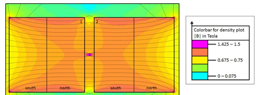
Fig. 2: Magnetic flux density  $|B|$  of two neodymium-magnets N48 (1 and 2), 2 mm apart, ferromagnetic wire (3) in between
