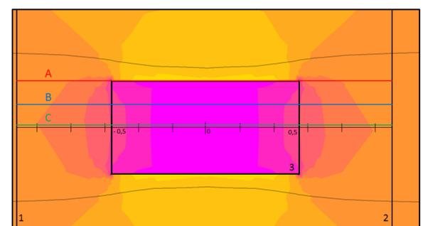
Fig. 3: Magnetic flux density  $|B|$  of saturated ferromagnetic wire (3) (0.5x1 mm) in the middle of two neodymium-magnets N48 (1 and 2), magnets 2 mm apart
