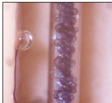
Fig. 6: Ferromagnetic beads in microchannel with applied magnetic field, picture of 1x1 mm
