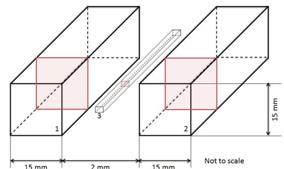
Fig. 1: Principle sketch of magnetic simulation, two neodymium-magnets N48 (1 and 2), 2 mm apart, ferromagnetic wire (3) in between
