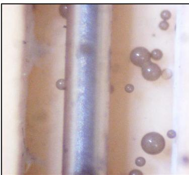
Fig. 5: Ferromagnetic beads in microchannel without applied magnetic field, picture of 1x1 mm
