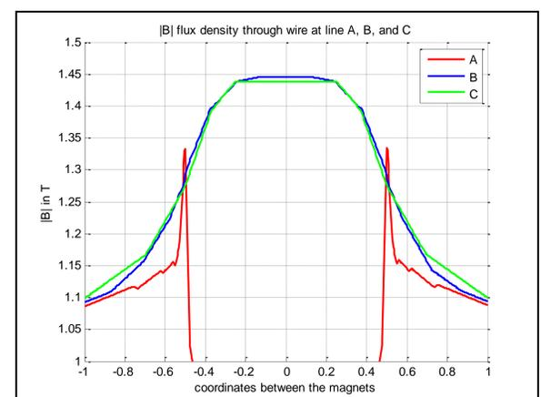
Fig. 4: Magnetic flux density  $|B|$  of saturated ferromagnetic wire (0.5x1 mm) at different section between two neodymium-magnets, magnets 2 mm apart
