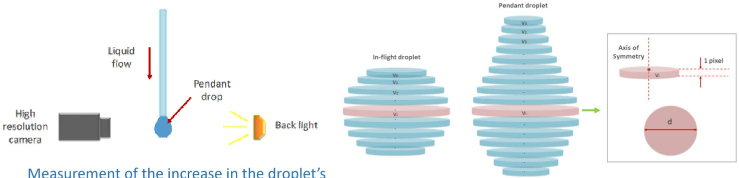
Measurement of the increase in the droplet's volume over time under a liquid flow
