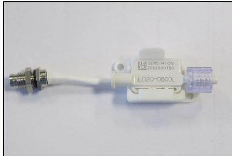
Flow sensor (Sensirion ) with its holder
