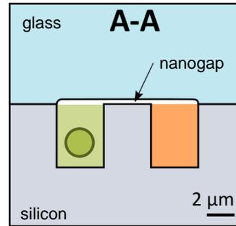
**reference- and detection channel:** 3 μm × 4 μm
