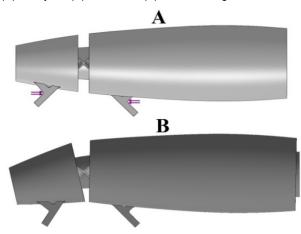
**Figure 2:** Mechanical behavior of total cast system (A) before and (B) after the external load is applied. An external closure mechanism applies a horizontal force (purple vectors) at each hook, creating a hinge-like reaction at the truss joint.
