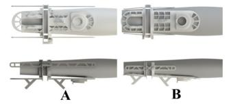
**Figure 5:** (A) original and (B) redesigned cast attachment. New design accommodates pediatric forearm dimensions, reducing gaps between padding and cast attachment components.
