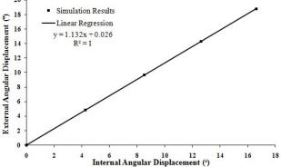
**Figure 4:** External versus internal angular displacement. Markers indicate calculated simulation values with a corresponding linear regression and an R<sup>2</sup> value of 1.
